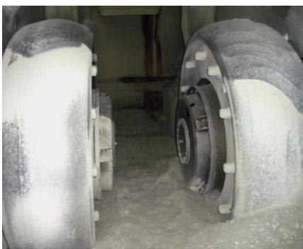
Fig. 1: Vertical roller mills are commonly used for raw material grinding due to their very good drying capacity.
