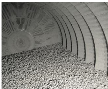
Fig. 2: Because of their reliability, ball mills still account for the majority of installed mills.
