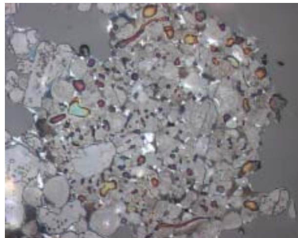
Fig. 2: Micrograph of a belite cluster with finely dispersed free lime in a phosphate bearing clinker
