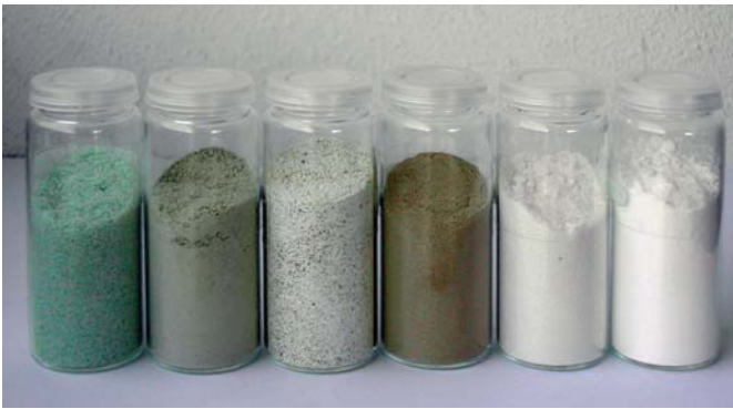
Fig. 1: Different solid reducing agents for chromium(VI) in cement. From left to right: Two iron(II) sulfate heptahydrates, two iron(II) sulfate monohydrates and two tin(II) sulfates
