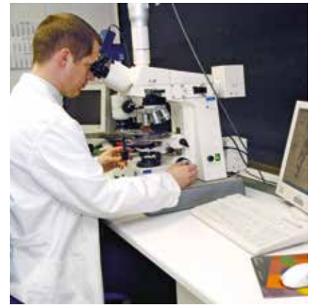
Figure 1: Clinker microscopy provided to support process optimisation of cement plants
