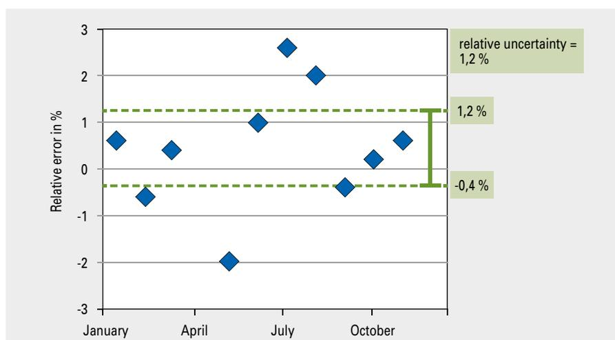
**Figure 2: Example of relative errors (blue) from regular scale checks of a belt weigher for metering clinker production and uncertainty assessment for the recorded annual clinker production (green dashed lines)**
