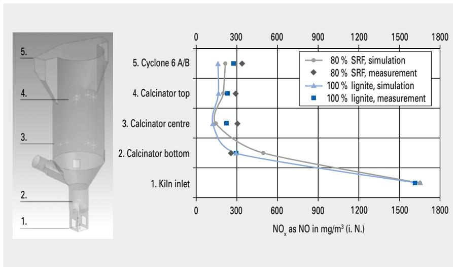
**Figure 2: Comparison of the measured and simulated NO<sub>x</sub> concentrations for 100 % lignite and 80 % AF utilization**
