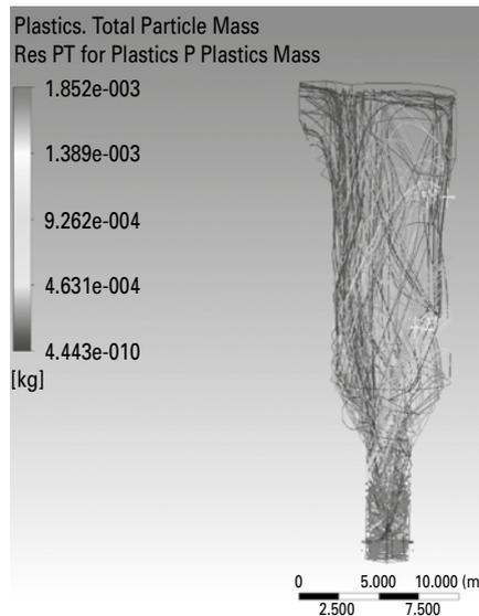
**Figure 1: Particle tracks of plastic materials from alternative fuels**
