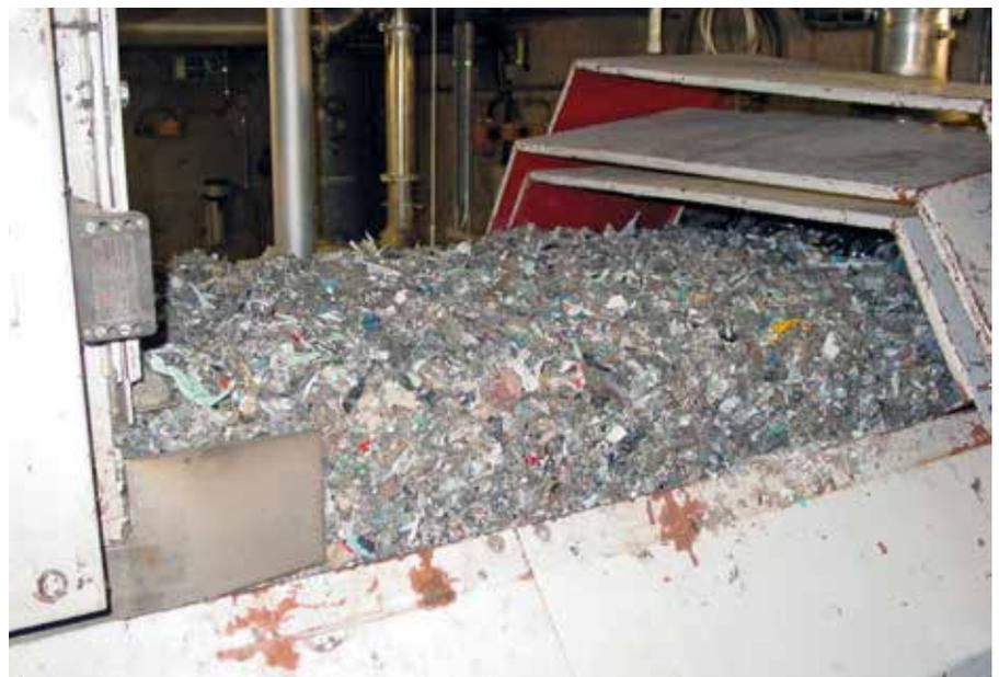
Figure 1: Belt weighfeeder for continuous weighing of alternative fuels
